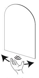
Your mirror comes with an infrared sensor located in the middie of the bottom. To activate the light and demisting pad, move your hand across the sensor once at a distance of around 5cm. To turn it off, move your hand across the sensor again.
